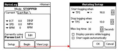
In this example, the scanner will automatically log when the TPS (throttle position sensor) is reading > 90%, and will continue to log until the TPS is reading below 10%, for a maximum of 30 seconds. To change which conditions start & stop the automatic logging, click the parameter name, the condition "<", or click on the value to type in a new one. You can also use the up & down arrows to "spin" the values up or down quickly.
